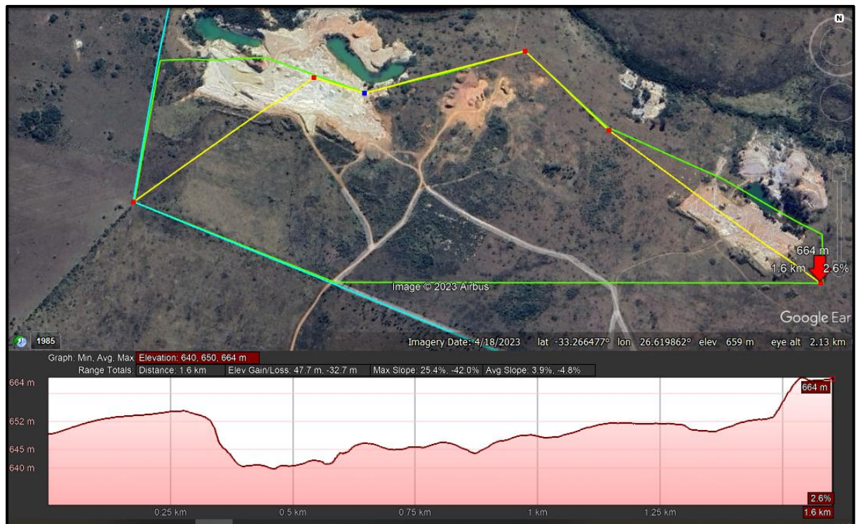
Figure 2: Elevation profile of the proposed mining area (image obtained from Google Earth).
